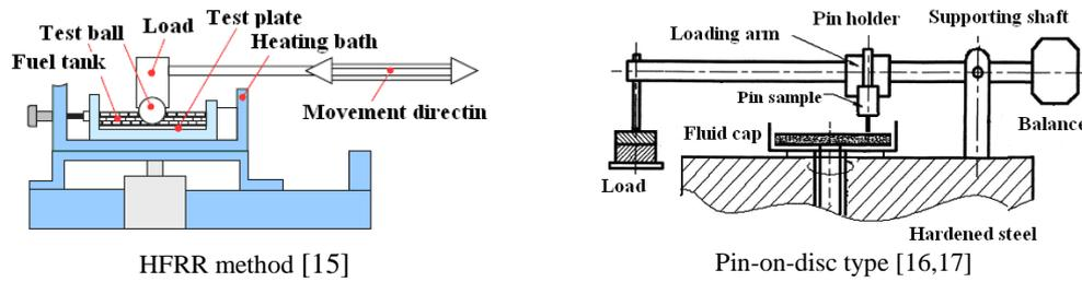
Fig. 1. Schematic diagram of wear testing rigs.
