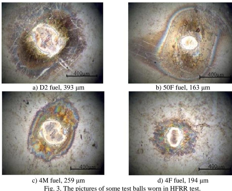
Fig. 3. The pictures of some test balls worn in HFRR test.
