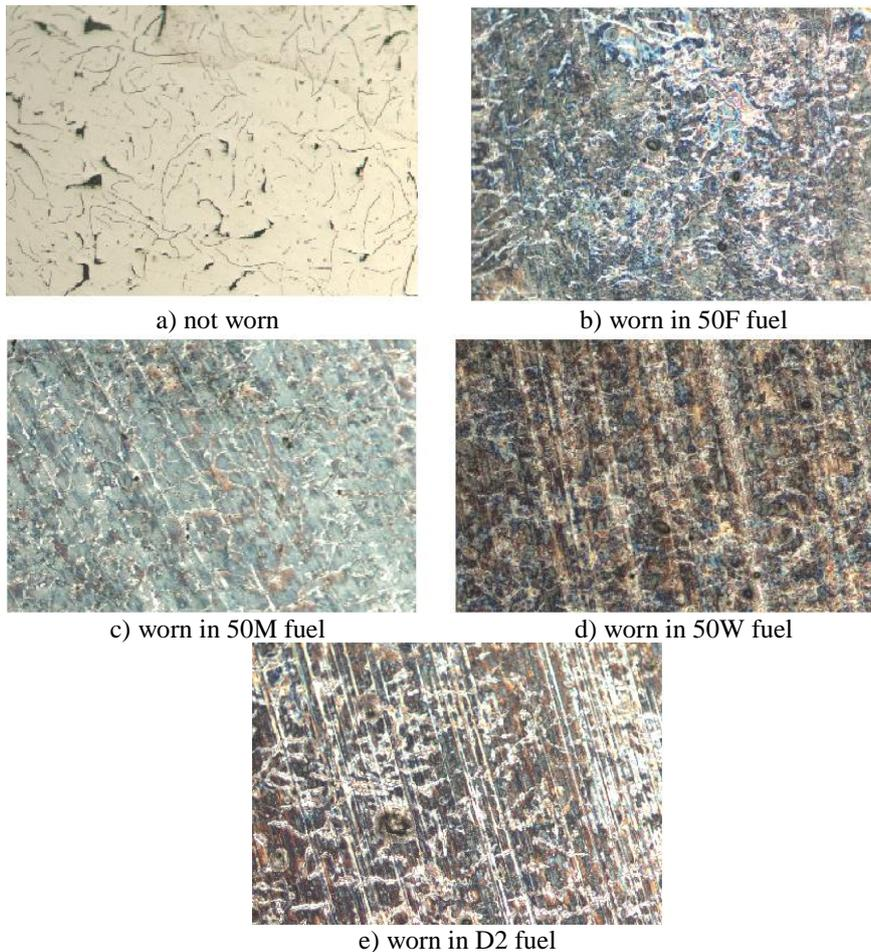
Fig. 5. Microscopic views of some samples worn in Pin-on-disc type wear testing machine.
