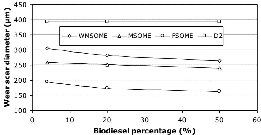
Fig. 2. Effect of biodiesel percentage on lubricity.
